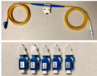
Emulated failures with optical attenuators tested under varying link speeds
